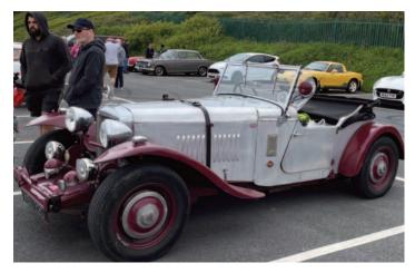
On investigation it turned out to be a TA14 chassis, wheels and radiator but not much else! The owner had battered the wings out of some steel he had lying around using what sounded like a hammer and a piece of wood and had made a pretty good fist of it. The car had an MGB engine and gearbox as the owner wanted something he could swap out easily when it failed - he clearly didn't understand Alvis' legendary reliability. Either that or he had no faith in his spannering skills
